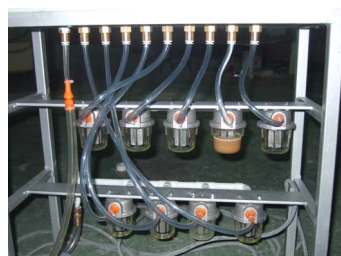
Figure 2. Odor generation unit: canister
