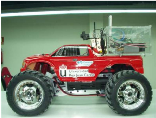
Figure 4. Finished prototype with the electronic circuits on a transparent box on its top.
