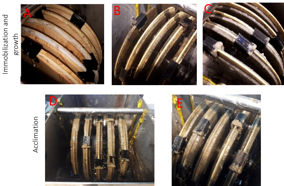
Figure 15. Evolution of biomass during the start-up of modified wooden-RBCs system: (A) Pre-treatment, (B) 31 days, (C) 57 days, (D) 71 days and (E) 80 days
