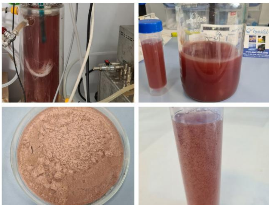
Figure III.7 Photos showing MPBR (top left), biomass collected at S2 (top right), lyophilized biomass (bottom left), and granulated biomass collected at P3 (bottom right).
