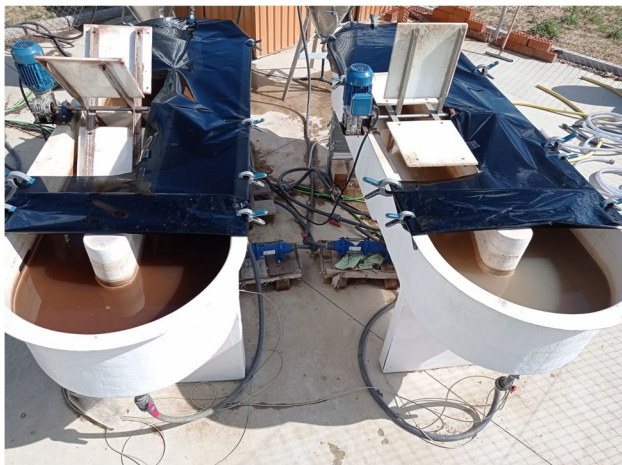
Fig. 1 Picture of the anaerobic raceway ponds operated in the University Rey Juan Carlos that were used as the source of biomass to inoculate the experiments (Móstoles, Madrid, Spain)
