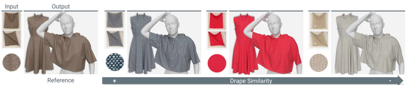
Figure 1: From just two depth images of a fabric sample casually placed in two specific configurations (input), we accurately infer the corresponding set of mechanical parameters of the material. Estimated parameters can be used in a cloth simulator, enabling to visualize the overall drape of any garment (output). Our method further introduces a novel perceptually-validated drape similarity metric, which enables sorting materials based on their final drape.
