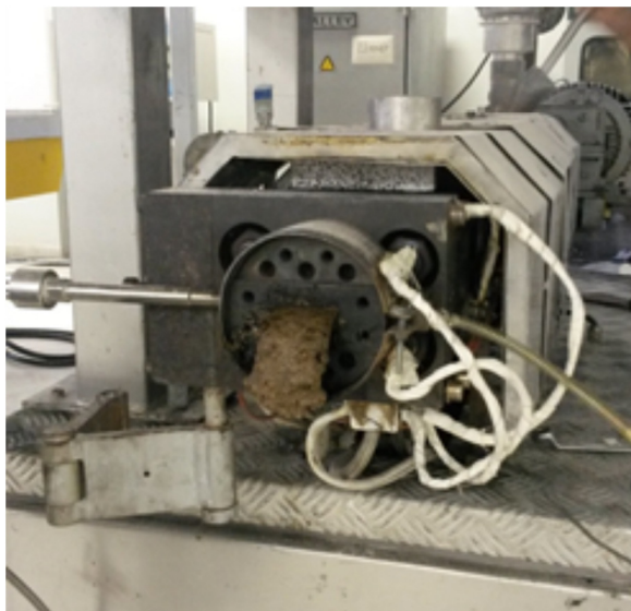
Fig. 1 – Co-rotating twin screw extruder adapted for high amounts of wood residue.
