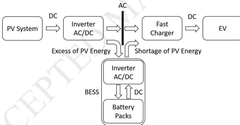
Fig. 4. Architecture of the off-grid PV-BESS studied.
