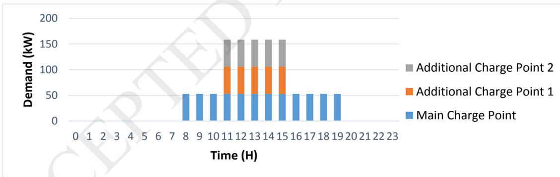
Fig. 9. Load profile of the improved case study
