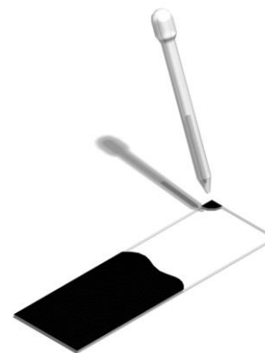
Fig. 1. Visual scheme of the solution deposition on cleaned glass substrate process.
